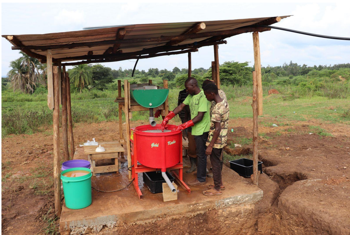
Figure 7: Gold Kacha without a sluice box located in Busia, Uganda, installed and operated by The Impact Facility throughout 2019 and 2020)
