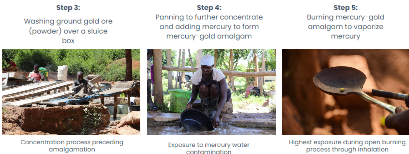
Figure 3: ASGM production steps: concentration and mercury amalgamation at ASGM site in Kenya.
