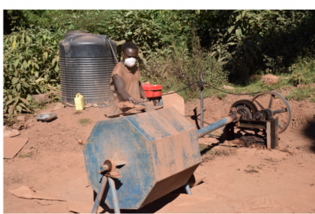
Figure 2: ASGM production steps: ore crushing and milling at ASGM site in Tanzania.
