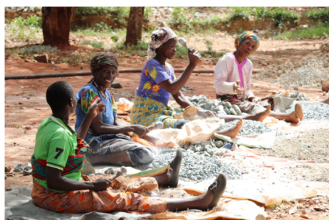
Figure 2: ASGM production steps: ore crushing and milling at ASGM site in Tanzania.
