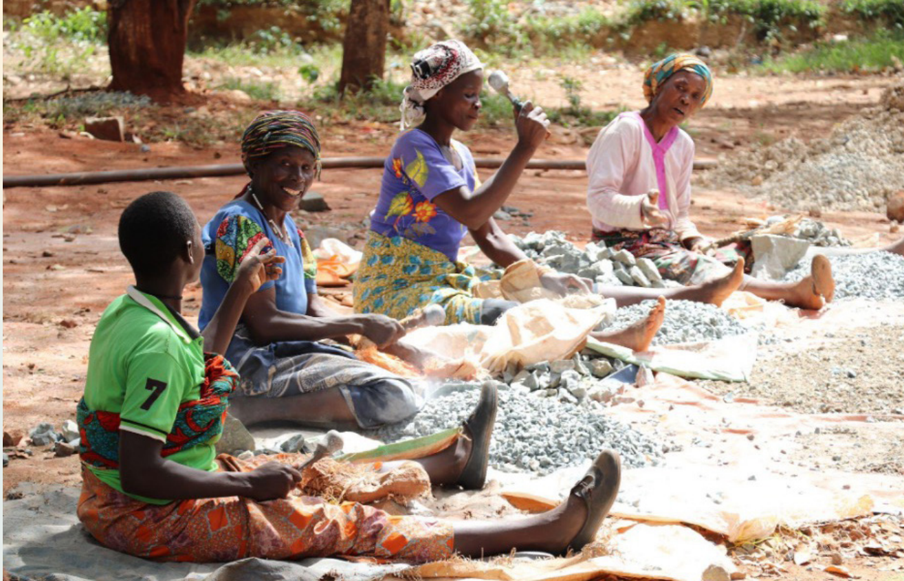
The initial crushing, hammering of the gold ore into smaller pieces before milling, is work largely reserved for women. They are typically paid a price per amount of ore they crush on behalf of other individuals.
