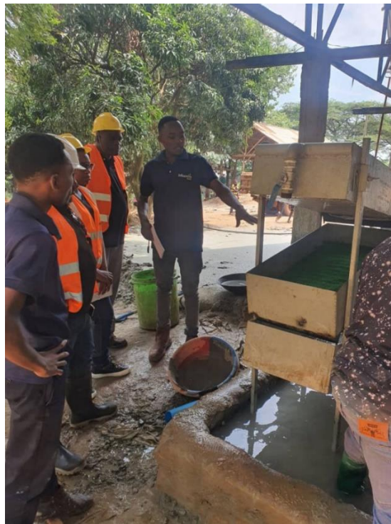
Figure 2: Testing of the High Banker Sluice at Nsangano Gold Mine.
