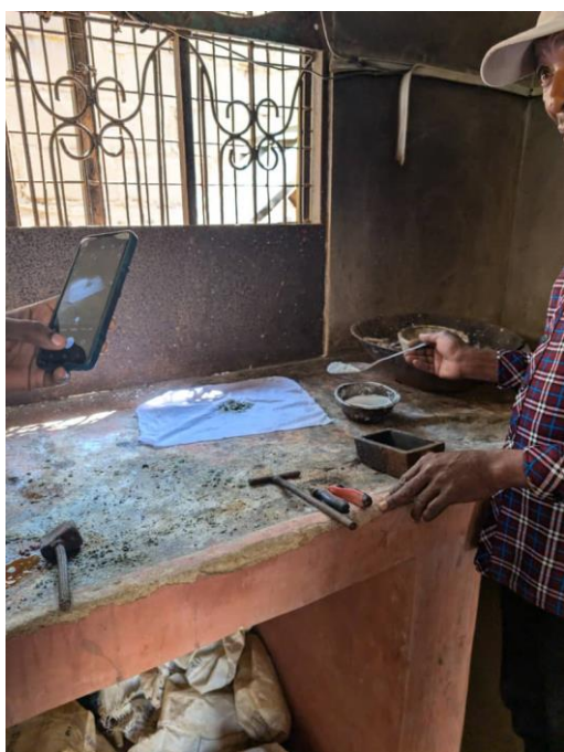
A. Mixing the gold concentrate and flux
