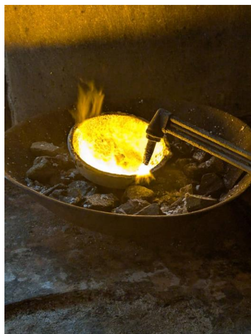
B. Smelting the concentrate – flux mixture
