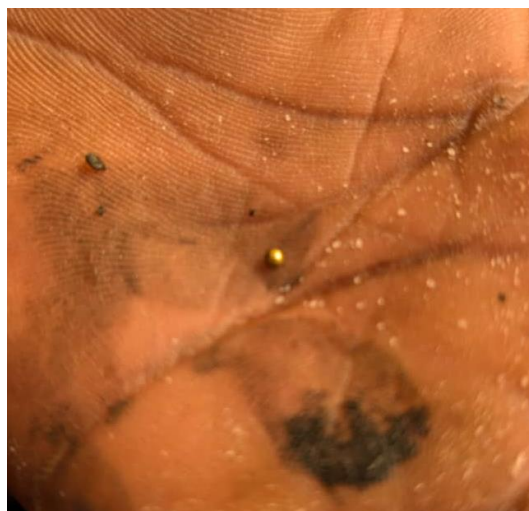
Figure 6: Gold Bead Recovered from the Direct Smelting Stage
